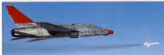
Above: Bullpup air-to-surface missiles could be fired from a number of modified F-100Ds. Some D-model 'Huns' were also wired to carry Sidewinder air-to-air missiles.
